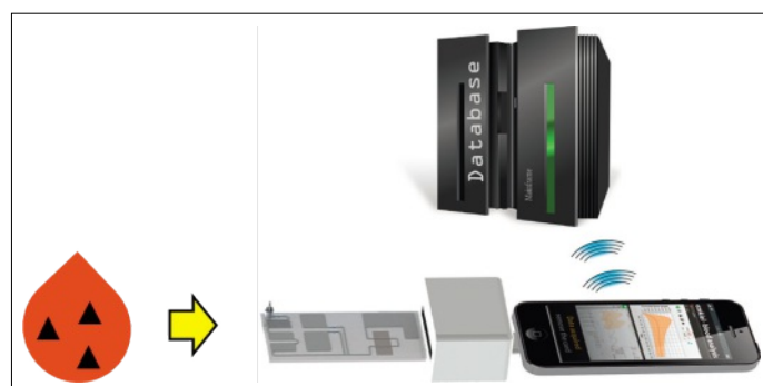
Design model of the future POC instrument for TDM. A drop of blood is processed in a disposable sample preparation cartridge. Analyte molecules – depicted as triangles – are then quantified in the analytical module before results are sent to a remote database. (Illustration C. Guiducci, EPFL, adapted by M. Pfeifer)
