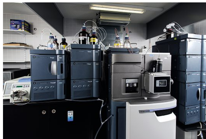
With the UPLC Xevo TQ-S researchers at the Inselspital Bern quantify known metabolites with a validated method. On the other hand, non-targeted metabolomics has the purpose to identify unknown metabolites. In this case, the scientists undertake a wide screening with the UPLC Synapt G2-S HDMS System in order to detect the maximum number of metabolites. (Picture Inselspital Bern)
