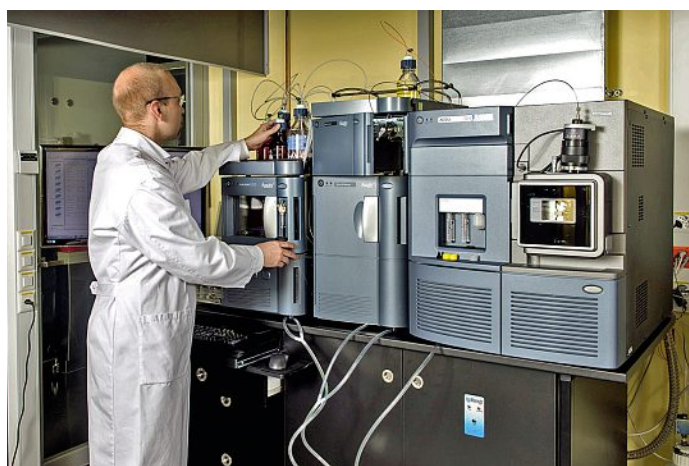
Acquity UPLC separation system coupled with a Xevo TQ-S (Waters) mass spectrometer at the Inselspital Bern. The UPLC separates metabolites, then the mass spectrometer ionises the molecules for the analysis. (Picture Inselspital Bern)
