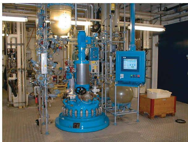
Fig. 9 The success of scale-up procedures for a large variety of hydrolase-catalyzed processes is based on robust, scalable and simple process designs without cofactor regeneration as shown here for a standard multi-purpose reactor for hydrolase-catalyzed desymmetrizations and resolutions using standard process control for the reaction and further processing and product isolation being performed at the bottom of the reactor in the lower level (Copyright @ Sigma-Aldrich).
