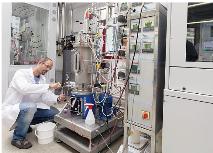
Fed-batch cultivation of Pseudomonas putida for the production of polyhydroxyalkanoates. (Picture photo-genic.ch)
