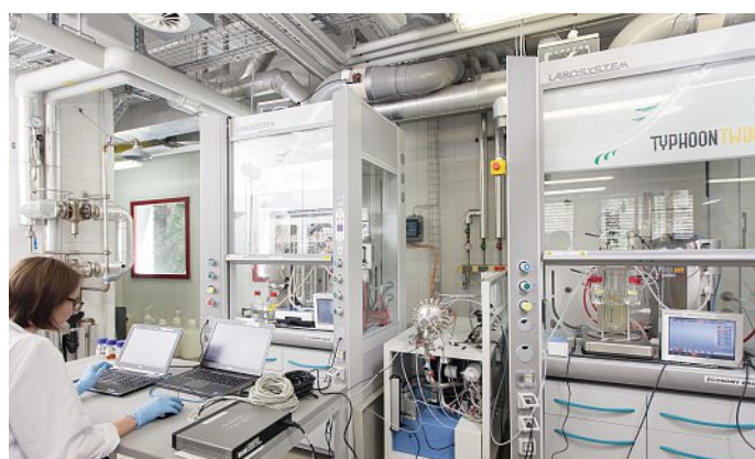
Safety first! The recently established fermentation infrastructure enables the safe handling of bioprocesses with dangerous gases (CO, CO 2 and H 2 ). (Picture photo-genic.ch)
