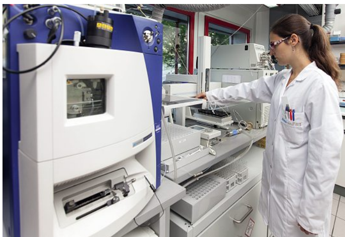
HPLC purification of synthetic peptides.
