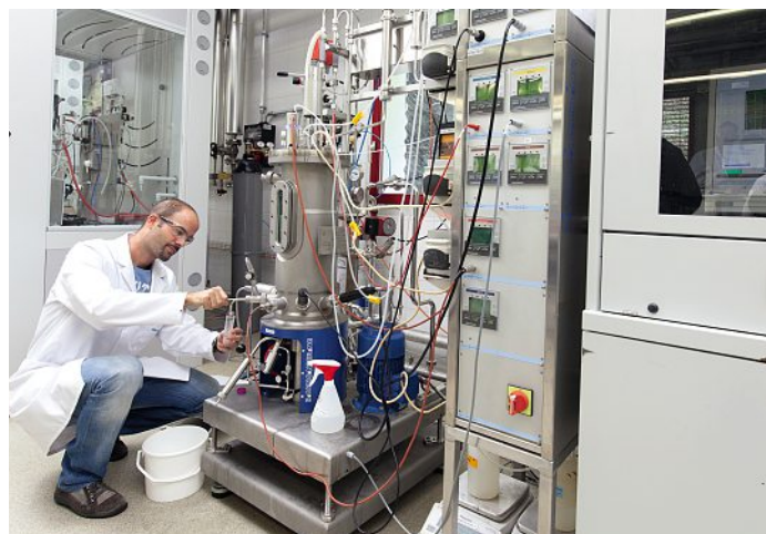
Fed-batch cultivation of Pseudomonas putida for the preparation of polyhydroxyalkanoates at HES-SO/Valais Sion. Photo: photo-genic.ch.
